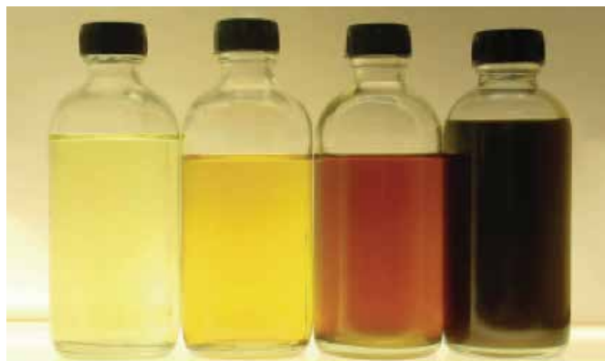
FIGURE 4: Progressive discoloration occurs when a heat transfer fluid is exposed to oxygen over time.
